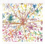
THE INTERNET, mapped on the opposite page, is a scale-free network in that some sites (*starbursts and detail above*) have a seemingly unlimited number of connections to other sites. This map, made on February 6, 2003, traces the shortest routes from a test Web site to about 100,000 others, using like colors for similar Web addresses.
